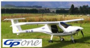
Modern carbon-composite aircraft optimised for pilot training and low-cost flying (LSA 600kg MTOW)
