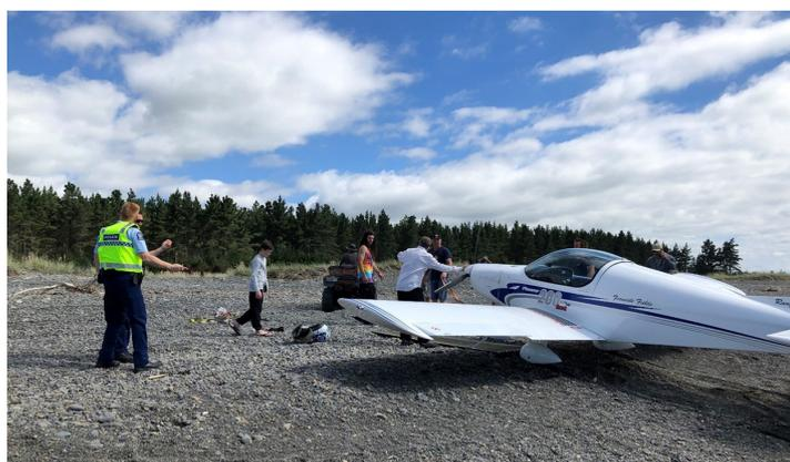
14th January 2022. Following a normal pre flight inspection, I departed NZFE and tracked east to the coast then turned north for Motunau Island. At 900ft overhead Ashley River mouth, I observed the cylinder head temperature gauge in the red, noting the engine sounded normal, I had power and the oil temp and pressure were normal, I reduced power and descended to 500ft for cooling. This
