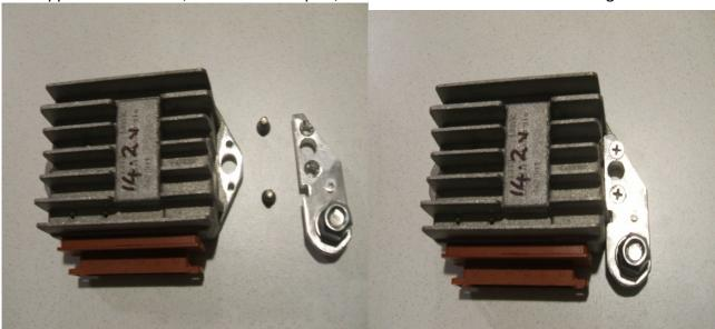
This regulator is a crude type which is either on or off (albeit at high frequency) so the battery is the primary smoothing component. Therefore, make sure the wiring is as thick and short as possible. The capacitor helps in this and should also utilise thick and short wire connections.
