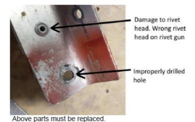
Above photos are from a typical CH 601 aircraft. Each CH design is different. Use your airframe model blueprints (drawings) and not the above examples for inspection and installation.
