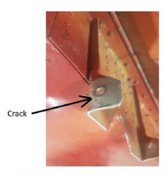
View of H.S. rear attachment bracket. A crack is developing in the part. Part must be replaced.
