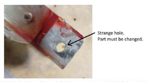
View of H.S. front attachment bracket. Bolt hole was not properly drilled. Part must be replaced.
