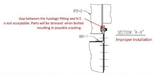
Above assembly drawing is for a typical CH 601 aircraft. Each CH design is different. Use your airframe model blueprints (drawings) and not the above example for inspection and installation.
