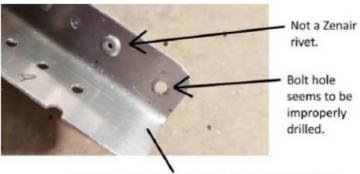
Bracket attaching horizontal stabilizer to fuselage. This is not an original bracket.
