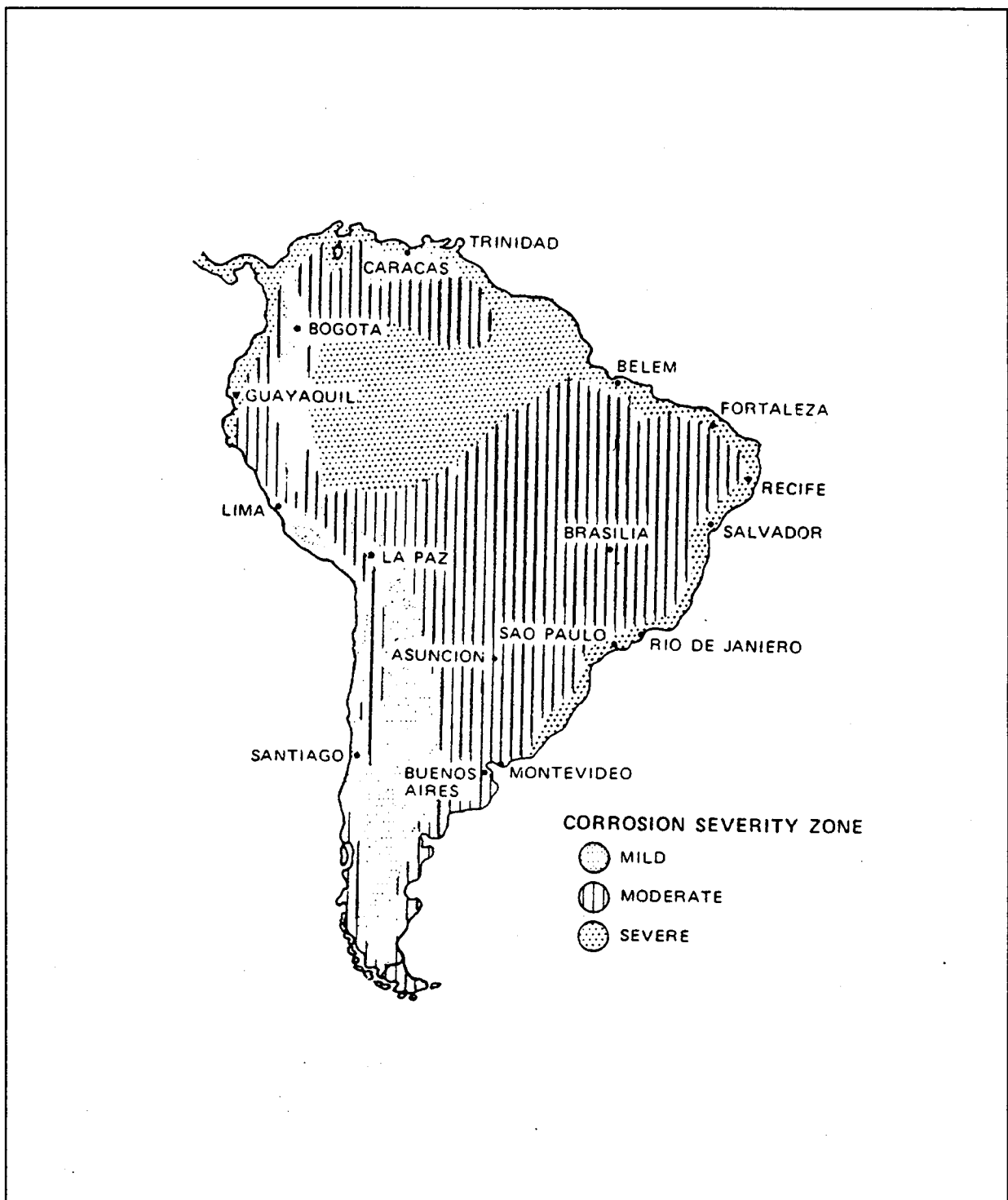
FIGURE 4-16. SOUTH AMERICA CORROSION SEVERITY MAP
