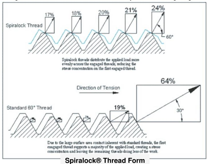
Spiralock® supply specialized taps to cut the threads and nuts with the specialized thread precut. For more information go to www.spiralock.com
