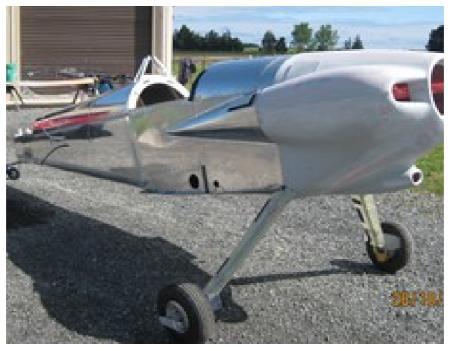
This latest project to hit the scene will be fully aerobatic rated at +6g and -6g capable of flying inverted and will have smoke on. The power plant is a fully reconditioned Continental 0320 rated at 160 HP. I believe that to this day there are currently about three of these models flying in NZ.
