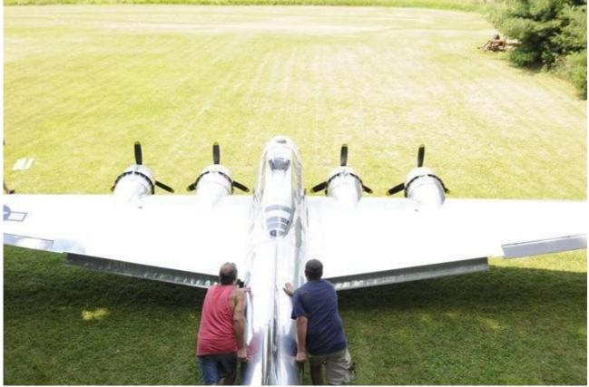
The project was started back in 1999 and is just now nearing completion. The airframe is all scratch built and made out of aluminium. The main gear retracts just like the real B-17 and has proven to be the most complicated part of the project.
