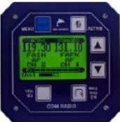
3.125" panel mount, only 5.5cm deep plus connectors, 250gm weight No knobs- easy to operate with gloved hands in open cockpit aircraft 10-28VDC 120mA Rx, 1.2A Tx @ 6W output
