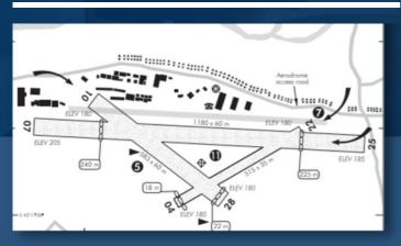
The above chart shows for Runway 25 shows a displaced threshold of 225 m. This allows foryou to pass safely over the top of any vehicles that are using the road adjacent to the Airfield boundary. It is very easy to become complacent in your local area if you perceive no risk.
