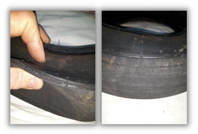
If your tires have been on for a few years, look hard to see if there is any split or cracks appearing. The pictures above are of a tire that was on an aircraft with an up to date annual, but the tire was shot. It looked ok from a distance apart from a bit bald but was about to go bang.
