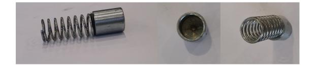
Note- this is the second recent NZ incident involving an AeroVee engine oil filter blow-out and subsequent oil loss. Other similar incidents have been reported in the USA with users correcting the defect by either a dowel insert in the existing piston to centre the spring, or using the aftermarket piston with a thicker wall to prevent the spring from cocking.
