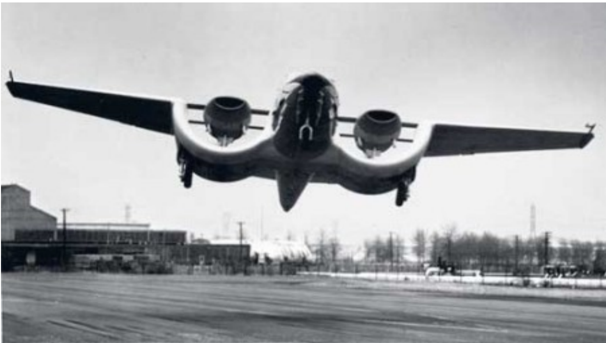
Custer Channel-wing: the original upper surface blown STOL aircraft
