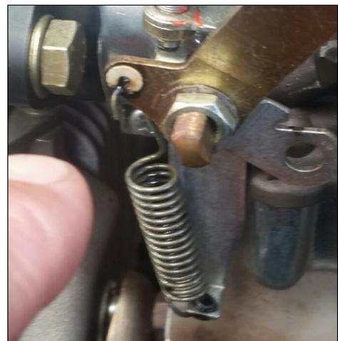
Another pic- these bushes are not installed on pre 2005 engines and I recommend installing them, but need to be inspected.
