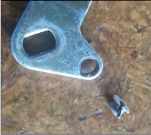
This is an arm of another customer's aircraft and at first look it appear good but on removal I find spring completely cut through bush,
