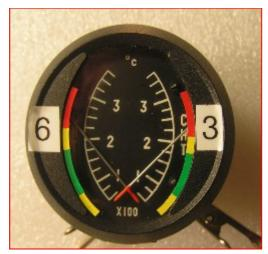
Alpi fitted a two channel cylinder head temperature gauge reading from 60deg to 360deg with sectors coloured green, yellow and red. The green covers 100deg to 180deg, yellow, 180deg to 220deg and red 220deg upwards.
