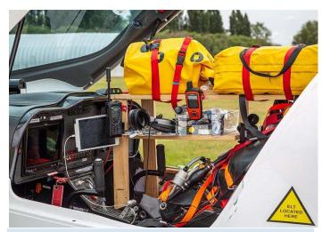
**Above**, nobody could accuse the flight of being unprepared! The top two yellow packages are the grab bag of emergency supplies on the left, and the life raft. Also visible are the Spidertracks and additional fuel tank. (**Aaron Murphy photo**)
